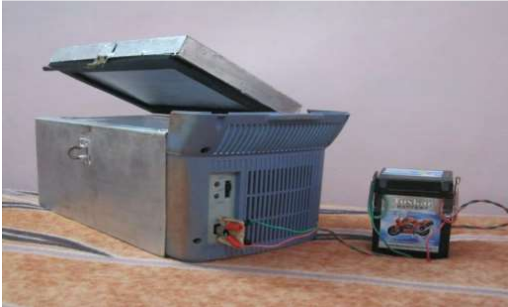
Fig 6.6: Fabricated model of the Thermoelectric Vaccine Preservator with battery attached.
